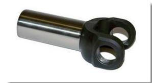
The entire forward end of the drive shaft is supported by the transmission **tailshaft bushing**, which is a press-fit into the **tailshaft housing**. This holds the output shaft centered and prevents runout (wobbling) and vibration.
