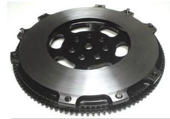
The flywheel is usually made heavy to give it a lot of mass. The momentum of the spinning flywheel helps to even out power pulses from the engine and provide smoother running.
