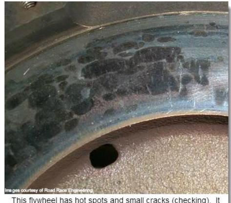
This flywheel has hot spots and small cracks (checking). It can probably be resurfaced.
