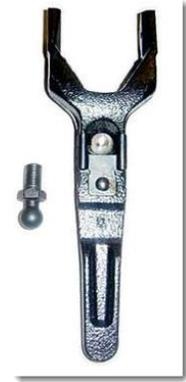
The fork extends through a hole in the clutch housing to reach the external parts of the release mechanism. A protective rubber boot fits in the hole to prevent contaminants and debris from entering the clutch housing.
