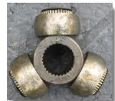
As with the outer CV Joint, the grooves, rollers and needle bearings are precision-machined to extremely close tolerances and hardened for long life. Molybdenum Disulfide grease is commonly used as a lubricant.
