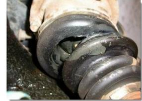
Other leaks can come from worn stubshaft (transaxle to halfshaft or wheel bearing) seals. Diagnosis should include careful inspection of the areas of the CV Joint outer races where the seal contacts for burrs and grooves. When in doubt, replace the CV Joint or halfshaft in question.
