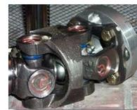
The Double Cardan design is not as prone to vibration due to rotational speed fluctuation as the single Cardan U-Joint. Rotational speed fluctuation is almost completely cancelled out because the Double Cardan design puts the yokes close together and at equal input and output angles.
