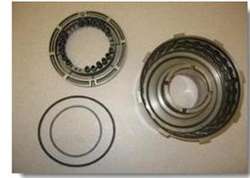
The multiple disc clutch housing can be either integral with the case or mounted on the input or output shaft. This allows for a sealing area for the piston seals. The clutch also includes a set of splines that mesh with the clutch disc and a system or sometimes a set of return springs for piston return.
