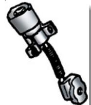
The **vehicle speed sensor (VSS)** is a permanent magnet signal generator that monitors vehicle speed, which is used in determining shift patterns and torque converter clutch applications.
