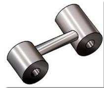
Front-wheel-drive transaxle and engine mounts can be inspected in much the same way as rear-wheel-drive transmission mounts. When the weight of the assembly is lifted from the mount, look for looseness or separation of the rubber from the metal. If the rubber bushing is loose on the mount bolt of the torque strut, the strut is defective.
