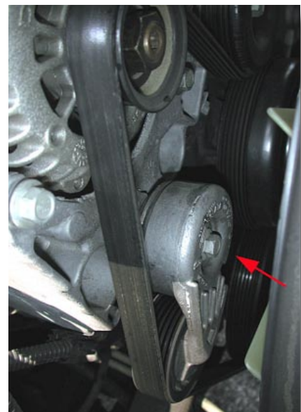
A Spring Applies Proper Tension
