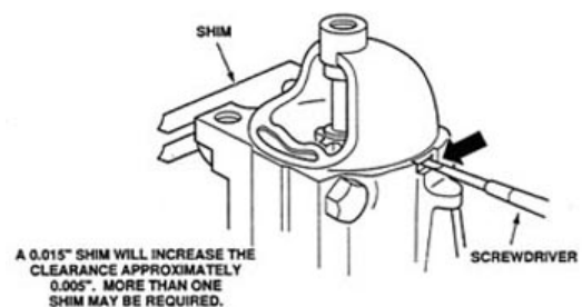
Flywheel to Pinion Clearance
