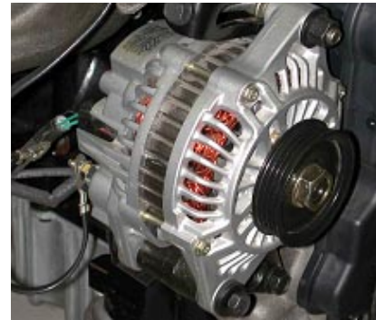
Modern AC Generator (Alternator)
