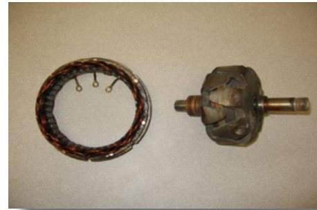
Alternator Rotor and Stator
