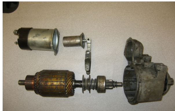
Internal Starter Components
